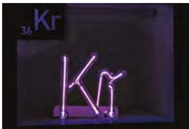
A discharge generated in a tube filled with krypton emits the violet light that is characteristic of it. (photo: Petr Jan Juračka)
