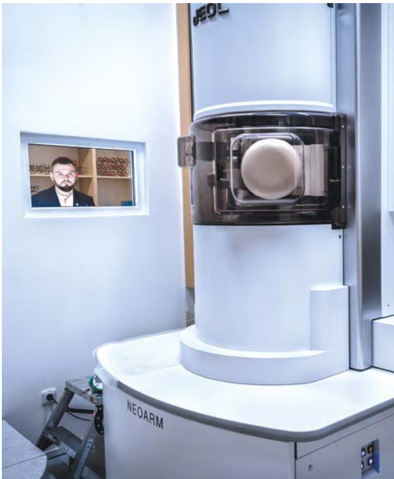
Michal Mazur at a JEOL NeoARM high resolution electron microscope, CUCAM project. (photo: Petr Jan Juračka)
