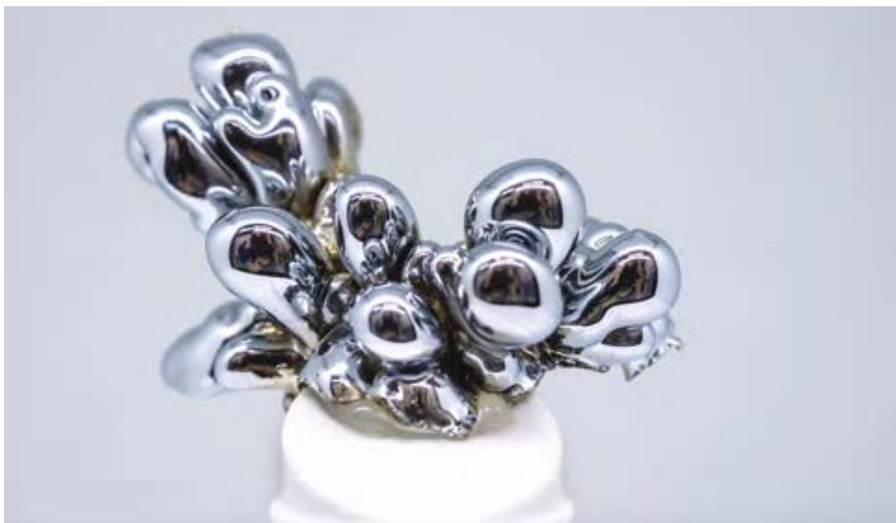
Chromium, which is visually one of the most attractive samples, was paradoxically created by chance during industrial chrome plating. (photo: Petr Jan Juračka)
