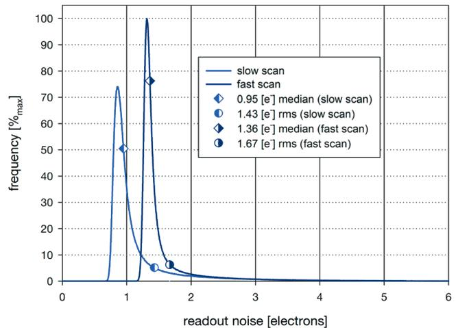
Noise distribution of the rms raw data values (noise filter off) of each pixel in the dark image of a pco.edge 5.5 at different readout speeds (slow scan / fast scan).
