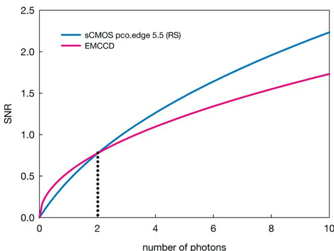
The graph shows the signal-to-noise (SNR) curves of a typical emCCD camera (gain = 1000) and a pco.edge 5.5 camera vs. number of photons.
